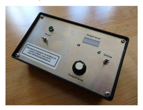
The *LL-PATCH* telephone interconnect is used for interfacing a dial-up landline telephone line (or fixed phone line) to a studio console, such as the Wantok-SBS-1 or SBS-2, or any other studio console or audio mixer. This permits the broadcast station to conduct live interviews or broadcast live feeds originating over the telephone network. Examples are field reporting and telephone interviews initiated at the studio.
